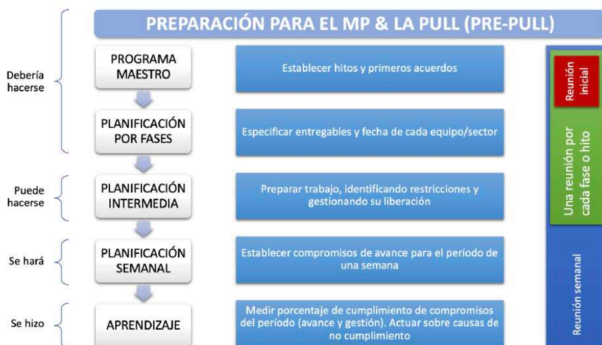
Fig. 29. Etapas del Last Planner System (por cortesía de THINK IN LEAN® by Juan Felipe Pons Achell).
